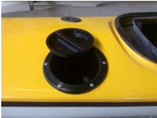
Day hatch installed on a Skua
